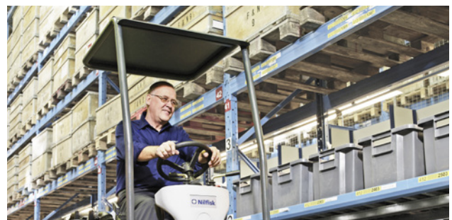
Overhead guard For additional operator safety, especially in warehouses and Industry
