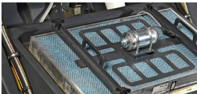
filters Paper filter: Works well in dry, high dust conditions Polyester: Excellent in moist applications, can be washed, dried and re-used
