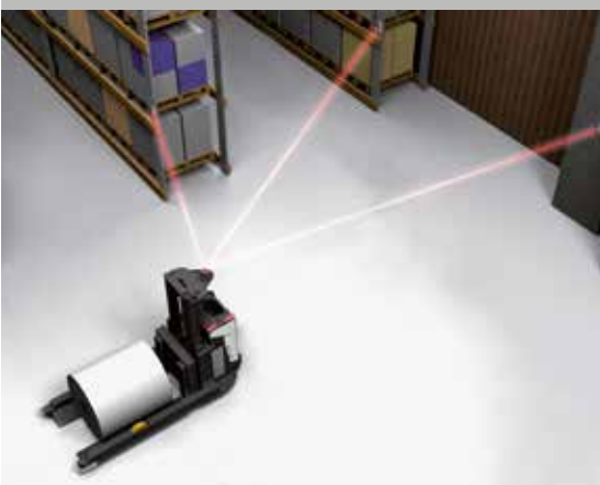
Laser triangulation (the most common)
