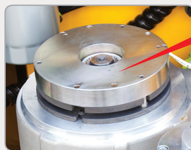
The electromagnetic brake controller is mounted on the traction motor.
