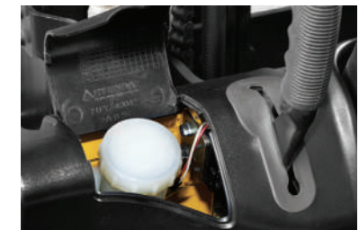
Brake oil reservoir with level sensor
